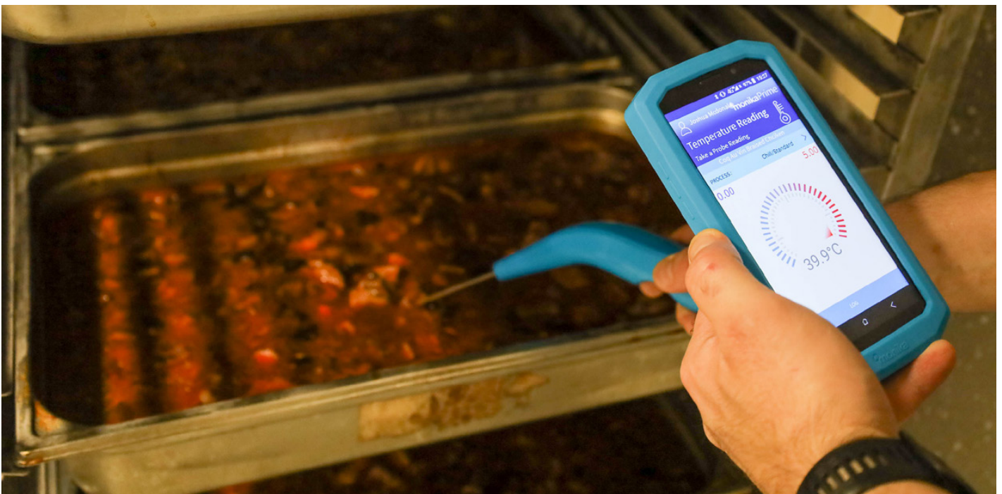
Pictured: A digital temperature probe used for automated logging of meat and meal temperatures
